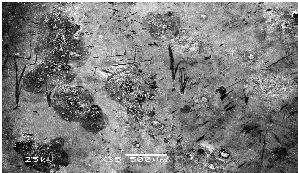
Figure 2. SEM micrograph (x 35) of the tinplate electrode surface in a synthetic solution after polarization from -1000 mV to + 1000 mV.
